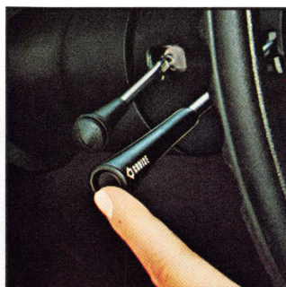
Automatic speed control (V8 engines with automatic transmission)
